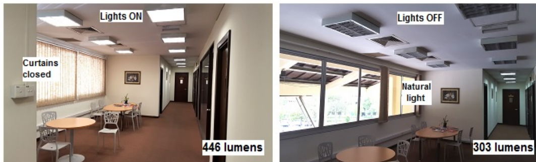
Figure 8: Concept of natural light and artificial light (HR block @ Admin building)
