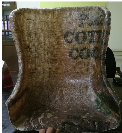
Figure 8. Biocomposite Go-Kart car seat
